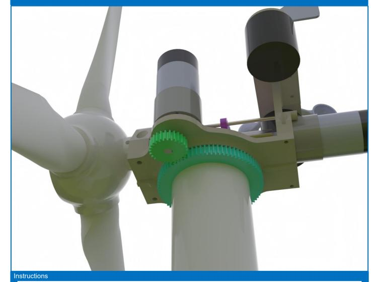
Assemble the nacelle's pivoting elements as shown in the figure. If necessary, refer to the CAD design.
